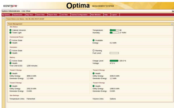
Optima Live View report for tower management module showing status of tower site
