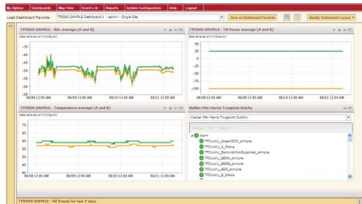
Optima dashboard displaying weekly Receive Signal Level (RSL), transmit power, internal temperature, and current alarm status for a microwave site
