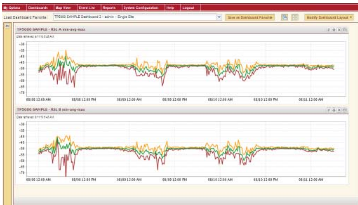
Optima dashboard displaying a microwave site's weekly RSL minimum, maximum, and average signal strength
